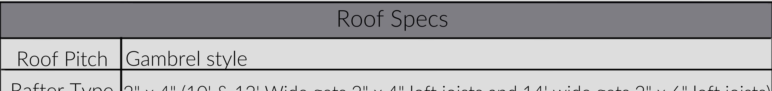
Rafter Type 2" x 4" (10' & 12' Wide gets 2" x 4" loft joists and 14' wide gets 2" x 6" loft joists)
